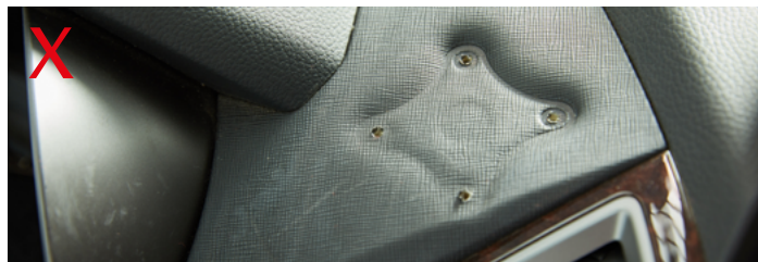
Holes in trim
