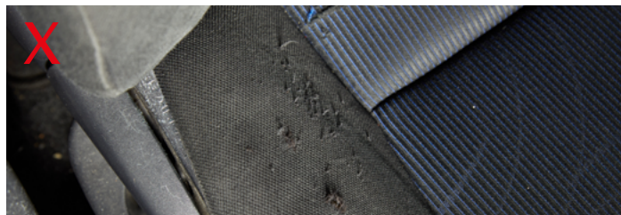
Excessive wear or rips in upholstery
